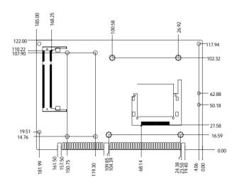
Figure 1.2: Board layout: dimensions (solder side)
